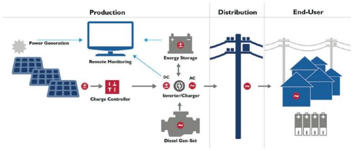
A decentralized power grid: that consists of completely off-grid Solar System, Battery Storage ESS, and Diesel Generators. Power is then distributed to units by transmission lines and managed by smart billing system. Suitable for remote areas.
